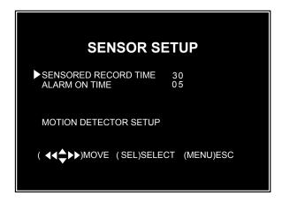
The Sensor Setup sub-menu sets how long (in seconds) the cameras will record once the sensor is activated, and whether or not, and how long (in seconds), the alarm will sound.
